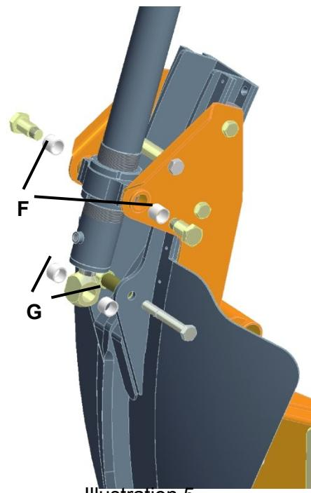
Unscrew bolts (D) and (E), remove worn bushes, insert new bushes (F) and (G).
