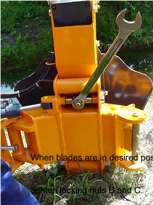
Locking nut C must be tightened
